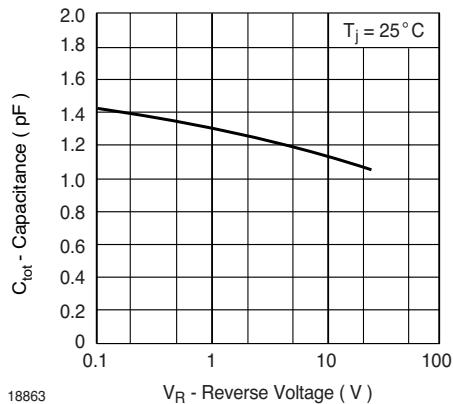
**Fig. 6** Capacitance vs. Reverse Voltage
