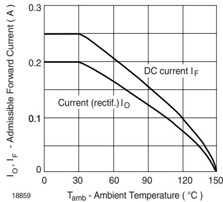
**Fig. 2** Admissible Forward Current vs. Ambient Temperature
