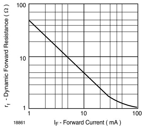
**Fig. 4** Dynamic Forward Resistance vs. Forward Current
